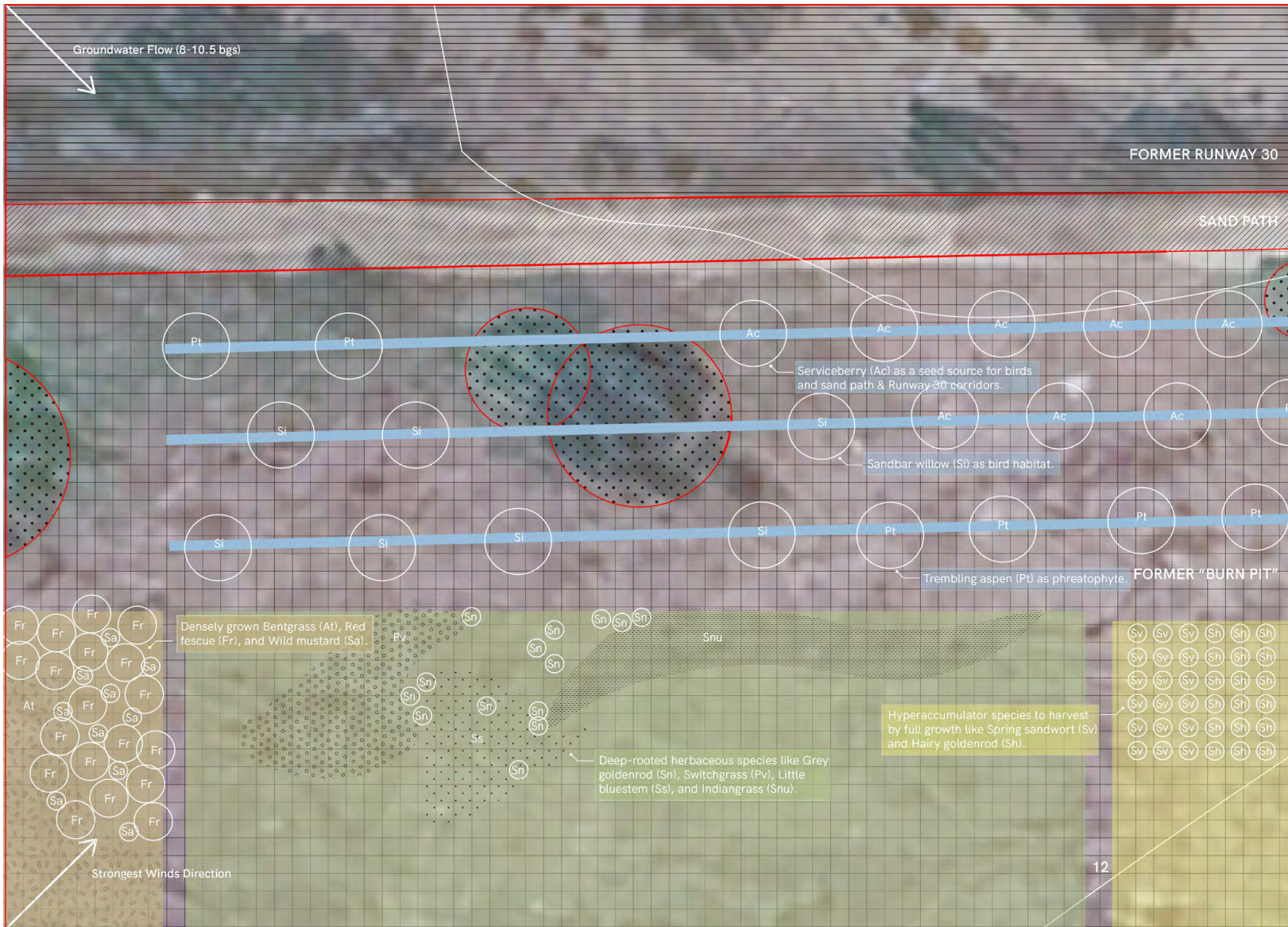
Vegetative Cover Detail Plan (1:10) w/ Phytoremediation Techniques
